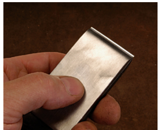
18 Hone the plane iron and install the cap iron so that it sits about 1/32 in. back from the edge.
