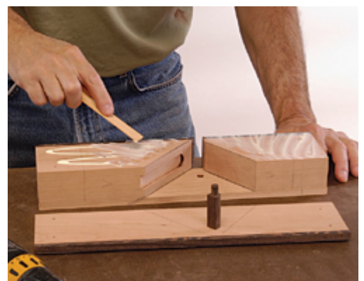
13 Spread glue and screw one cheek to the blocks. Then, add the pin and join the other cheek.
