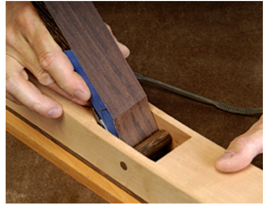
17 Test the wedge in the plane. Sand the surface to achieve a snug fit against the crosspin.
