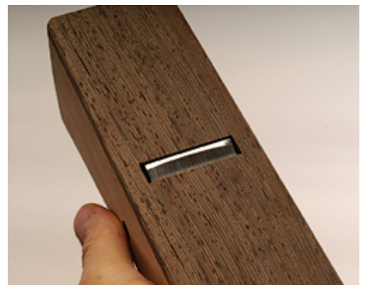
19 Install the iron parallel to the sole. Tap to increase depth. Tap back of plane to reduce cut.
